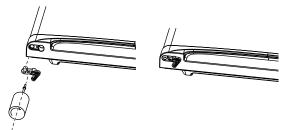
17 Install the freezer compartment door, then install the upper hinge and the left side upper hinge cover (found in accessory bag) on the top left side of the refrigerator.
