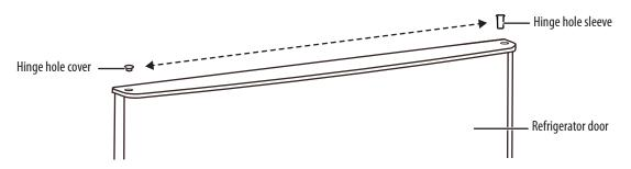
**9** Remove the screw hole covers from the center left side of the refrigerator and install them in the center right side of the refrigerator.
