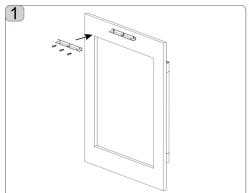
1. Fix the connecting plate to the corresponding hole in the wooden door.
