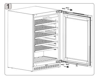
1. Remove the screws holding the hinges from the box and set the door aside.
