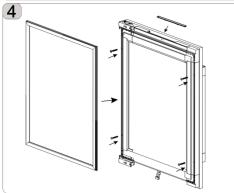
4. Use 4 long black screws to drive through the door from inside of the glass door into the wood door.
