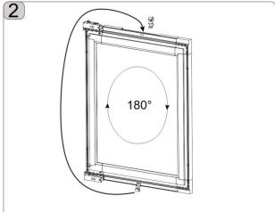
2. Remove the induction magnet unit from the bottom of the door and secure it to the other end of the door.
